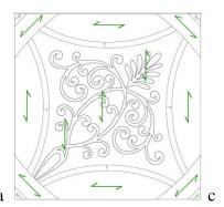
Fig. 6. Tile from the Boucher Room and the Corner Salon (a - tile view, b - design and fibre direction).
