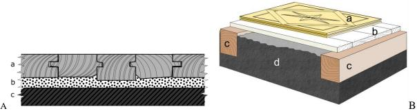
Fig. 9. Manner of flooring installation in the Chapel (A: a - tile, b - sand, c - concrete) and the manner of flooring installation in the Ball Room (B: a - tile, b - boarding, c - ceiling beams, d - sand)
